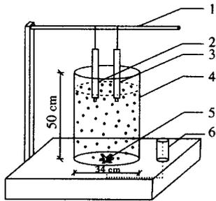
Fig. 2. experiment equipment. 1. bracket 2. OBS-3A 3. LISST-100 4. cylindrical cell 5. impeller and 6. electromotor.
