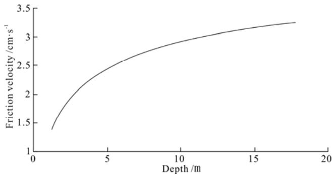
Fig.3 Distribution of friction velocity of tidal flow
