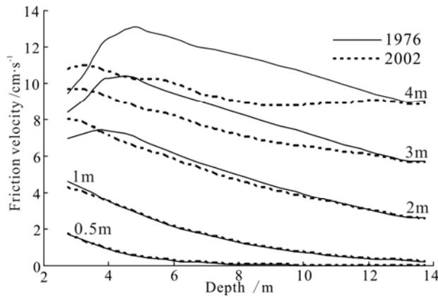
Fig.4 Distribution of near-bed wave generated friction velocity
