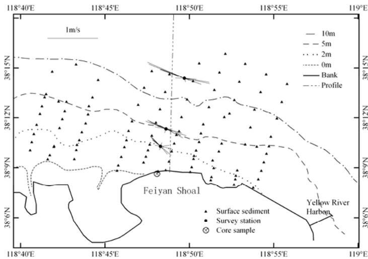
Fig. 2 Vector graph of field tidal flow and survey sites in the Feiyan Shoal
