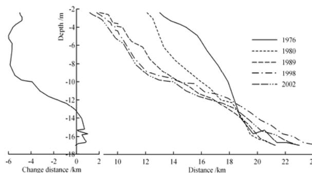
**Fig.6 Erosion of coastal profile and corrosive distance**
