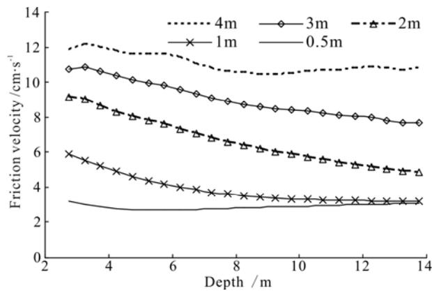
Fig.5 Distribution of tidal and wave co-action generated friction velocity
