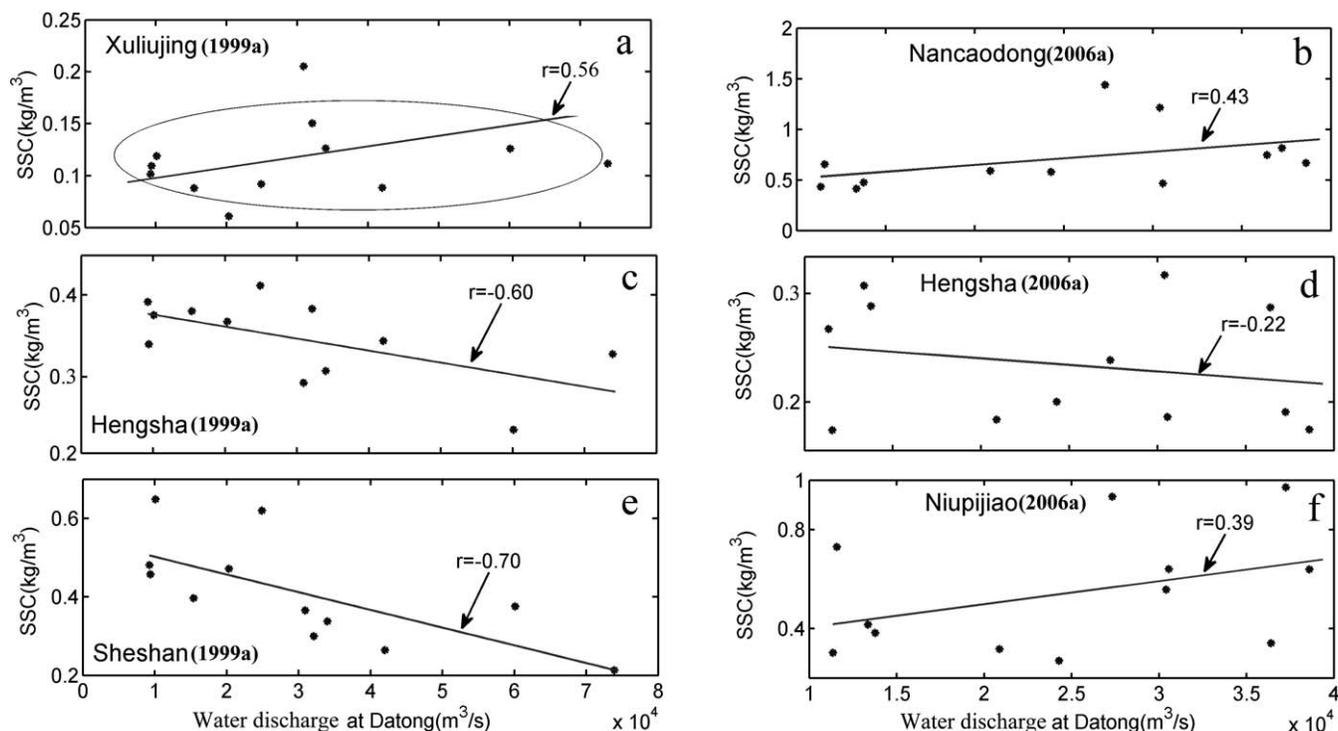
Figure 5. Relationships between the discharge at Datong and the SSC at the other station.
