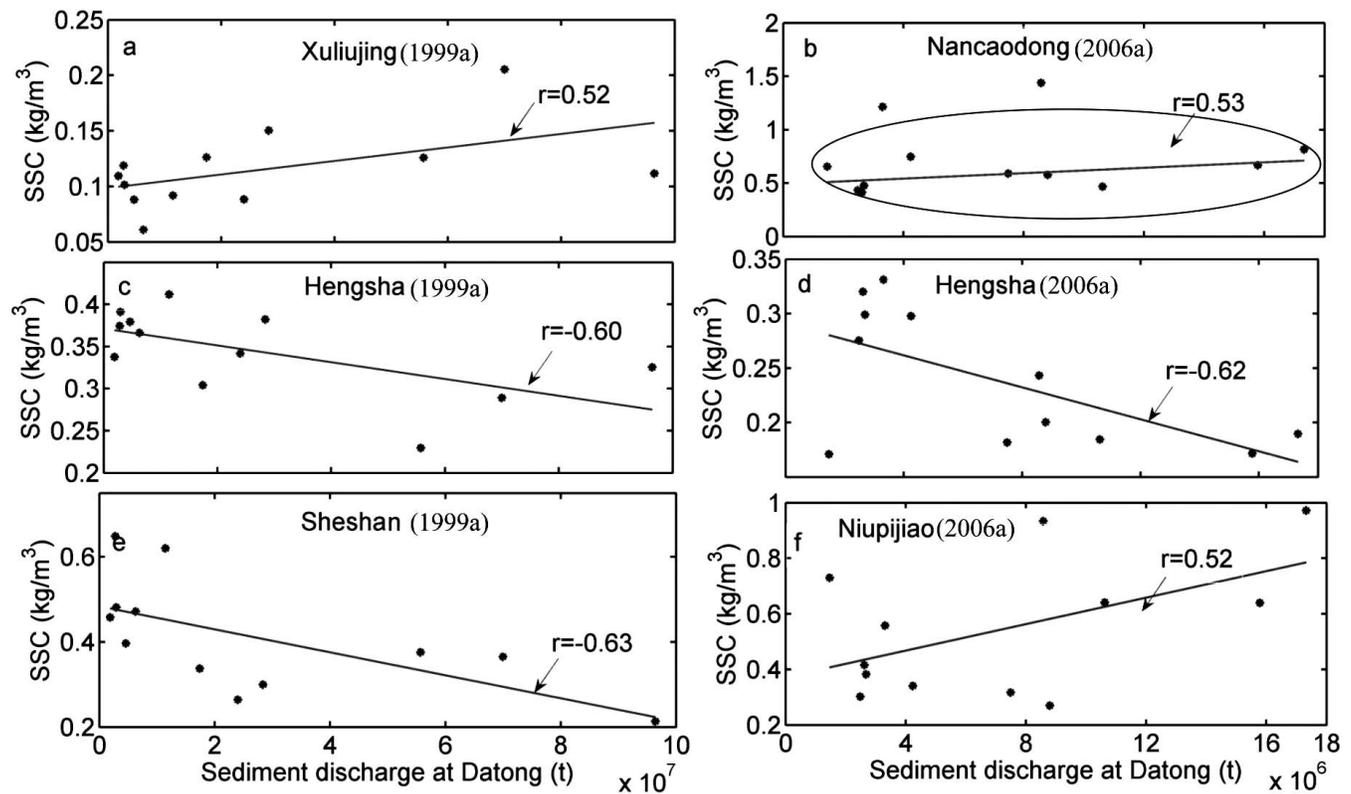
Figure 6. Relationship between the SSD at Datong and the SSC at the other station.
