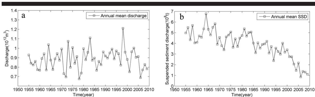
Figure 2. Annual discharge and suspended sediment discharge at Datong.
