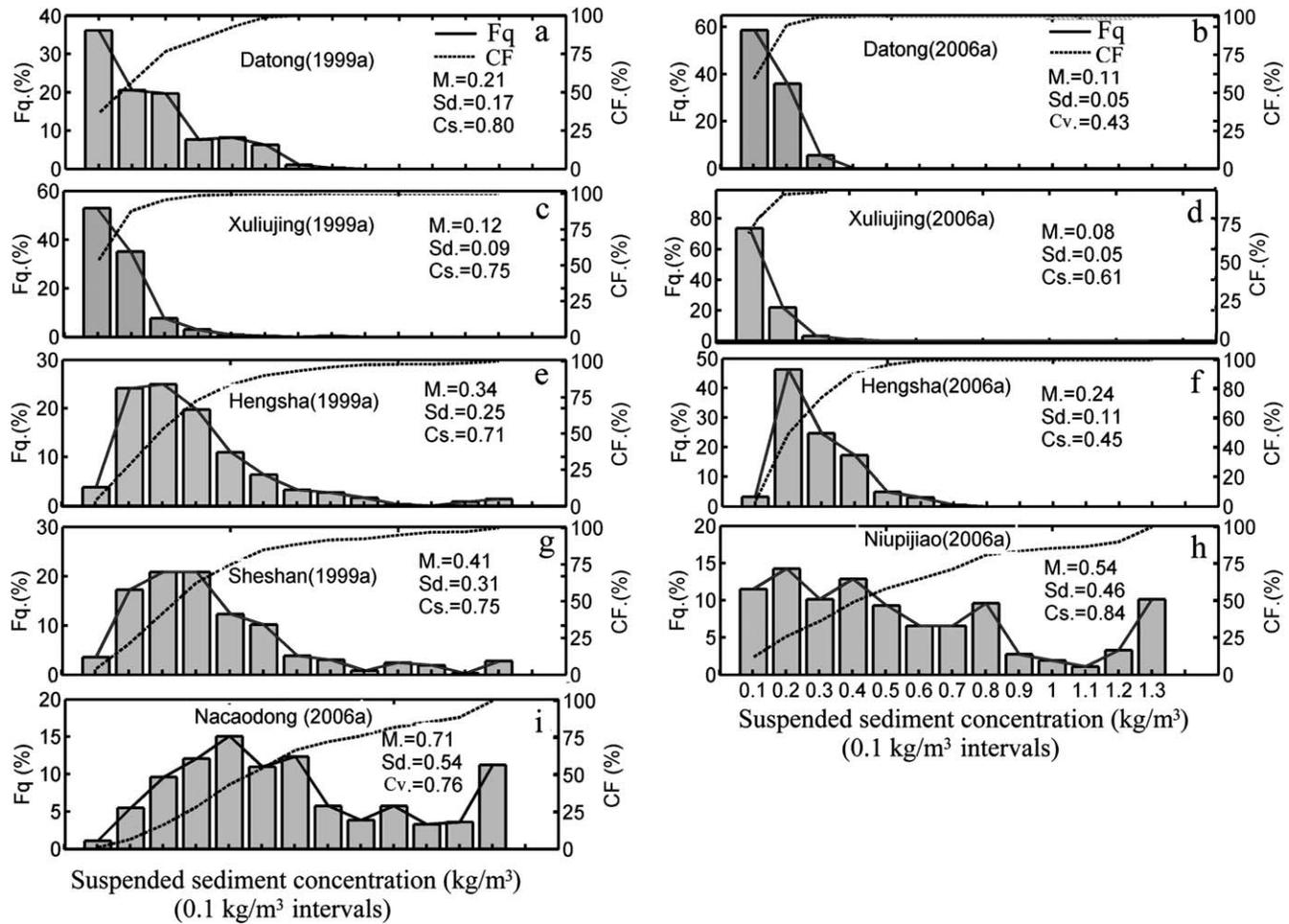
Figure 4. SSC occurrence at stations in 1999 and 2006 (Fq: frequency curve; CF: cumulative frequency curve; M: monthly mean; Sd: standard deviation; Cv: variation coefficient,  $Cv = Sd/M$ , representing the deviation of the SSC from the monthly mean).
